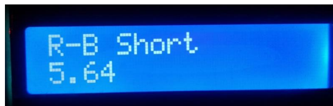
Fig 5.4 RB Short Fault Distance in Kilometer
