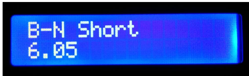
Fig 5.13 BN Earth Fault Distance in Kilometer
