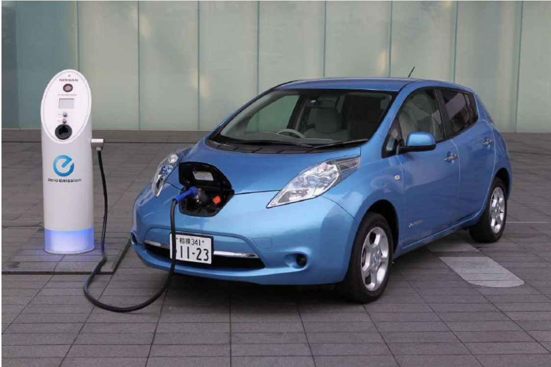
Fig. 2.11 External look of Nissan Leaf in charging mode [55].
