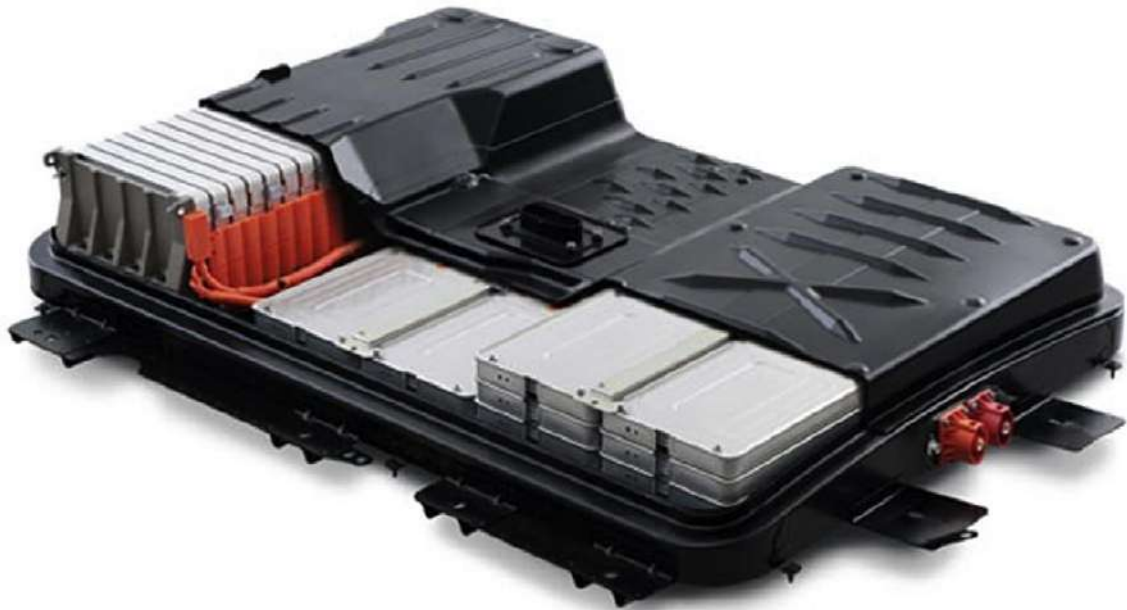
Fig. 2.12 The 24 kWh Nissan Leaf Li-ion battery pack with AESC Li-polymer cells [55].
