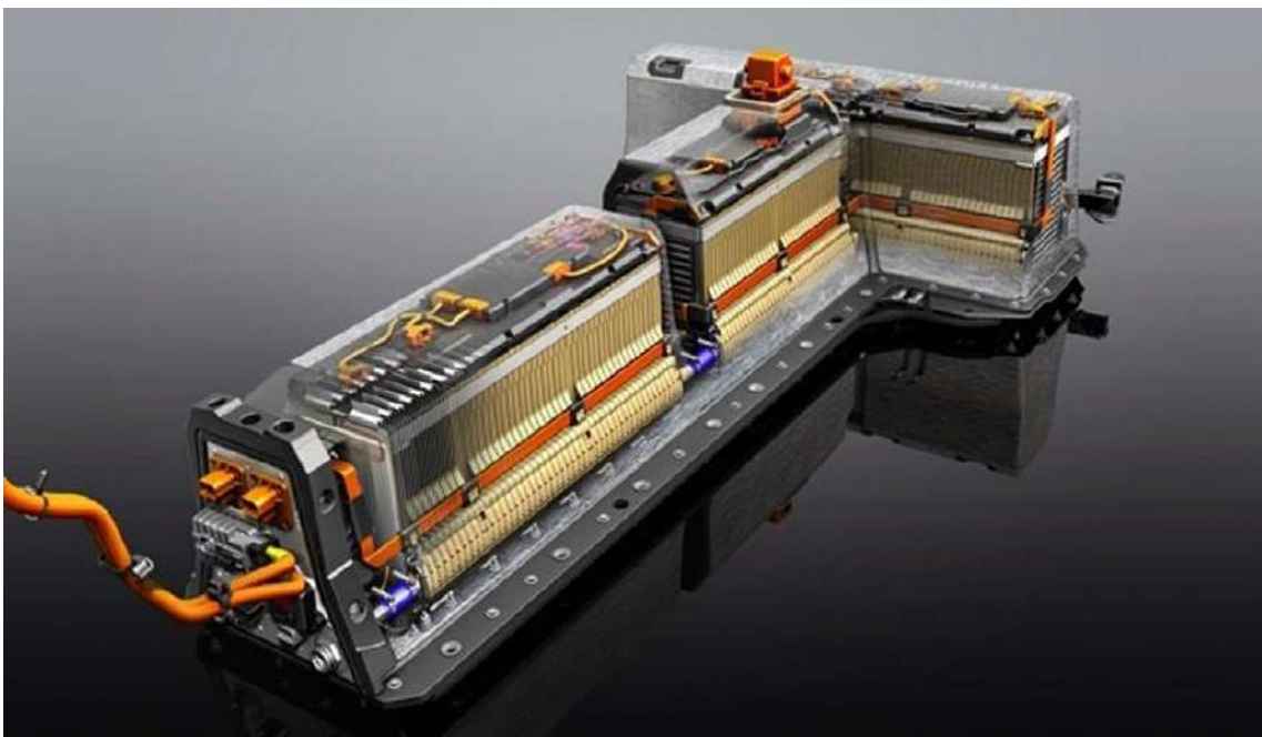
Fig. 2.13 The 16 kWh Chevrolet Volt Li-ion battery pack with LG Chem Li-polymer cells [55].
