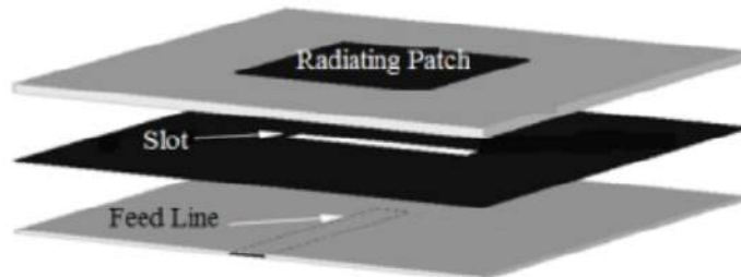
Figure 1.12: Aperture coupling feed [18]
