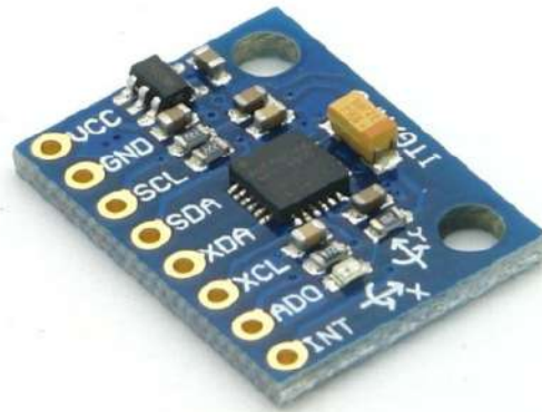
Fig. 3.2 MPU6050 Accelerometer and Gyroscope Module [41]
