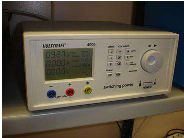
Figure 3.7 An adjustable switched-mode power supply for laboratory use [36]
