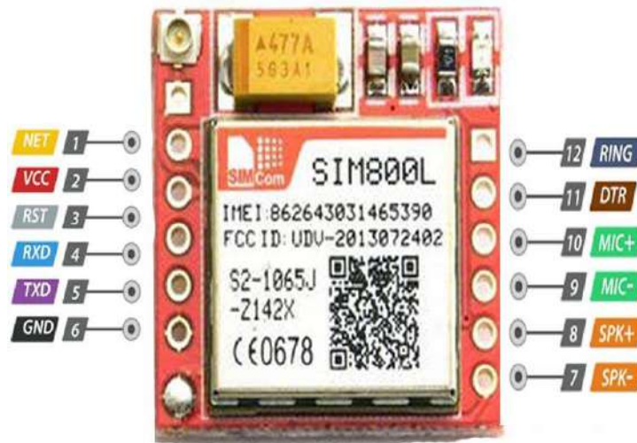
Figure 3.6 SIM800L Diagram of Pins [35]
