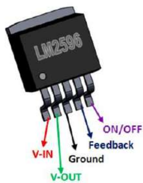
Figure 3.4 Diagram of LM2596 IC Pins [34]
