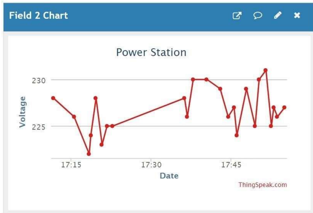
Fig. 4.6. Output of the device in the cloud platform (Voltage)
