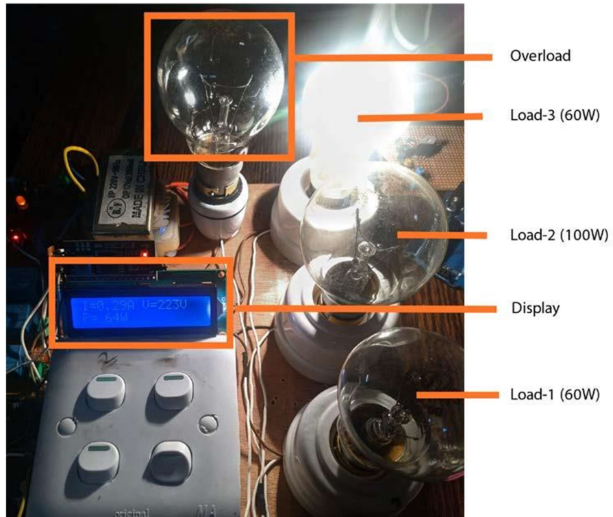
Fig. 4.2. LCD Display View (Load-3 Active)
