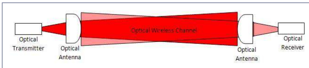
Figure 1.7 The light divergence increased by Optical Antennae
