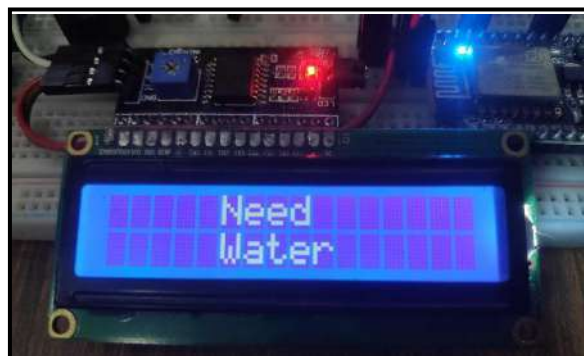
Figure 8(a): The "Need Water" message is displayed as the hand moves to the left side.
