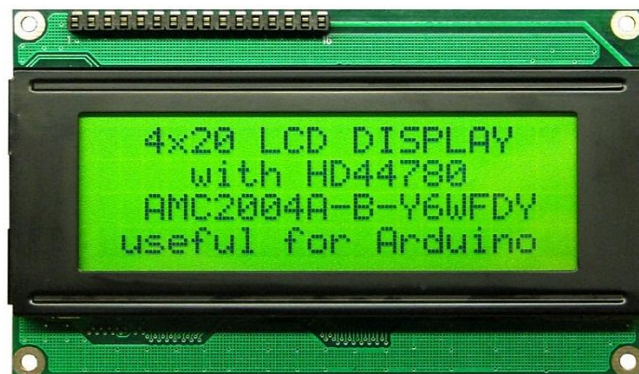
Fig. 3.15 Physical view of LCD 20x4 [19].
