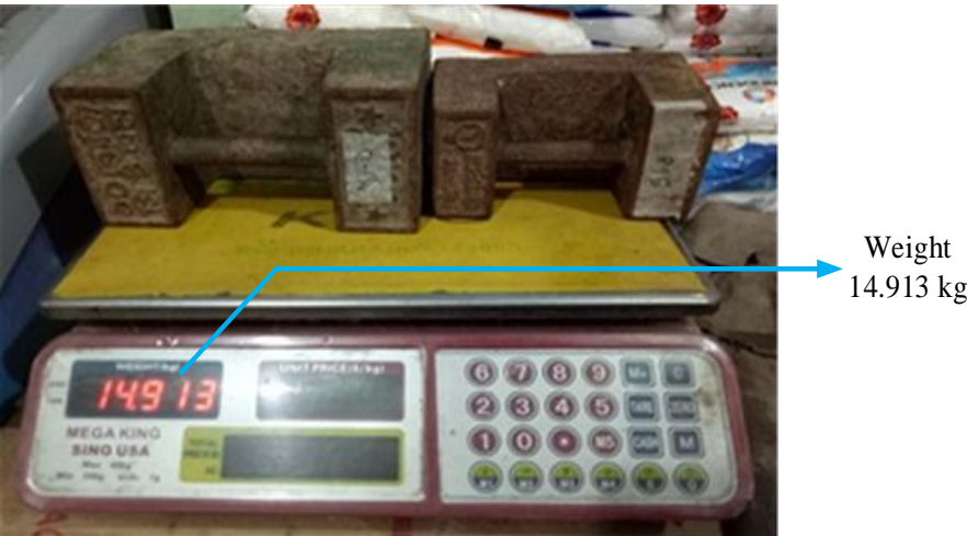
Fig. 5.4 Weight measurement in commercial weighing machine.
