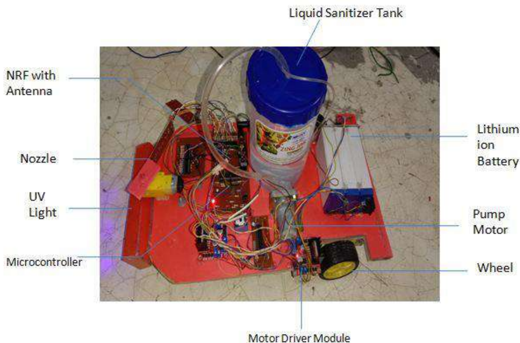
Fig 5.3: Receiver Portion and Prototype of the Robot
