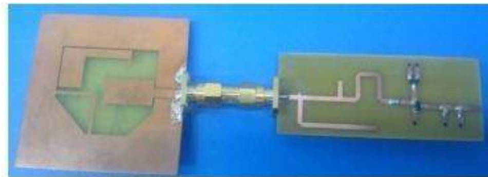
Figure 4.10: Photograph of the fabricated antenna of [158].
