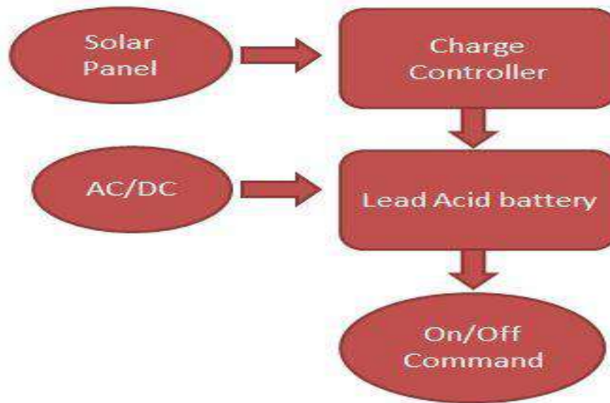
Fig. 3.3: Power System block diagram of designed solar car
