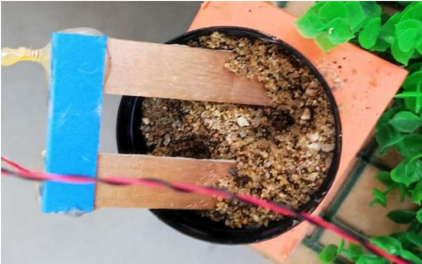
Fig. 5.3.4: Soil Moisture Sensor
