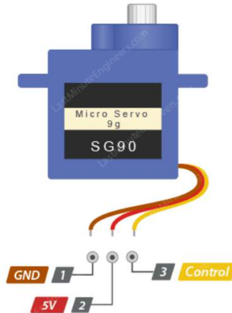
Fig 3.16: Pin diagram of Servo motor SG90 [17].
