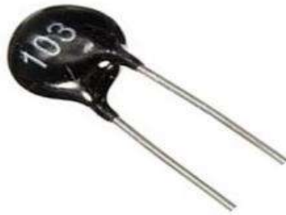
Fig. 3.6 NTC Thermistor (10Kohm) [24]
