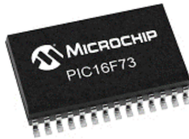
Fig. 3.1: Photography of PIC16F73 Microcontroller [5].
