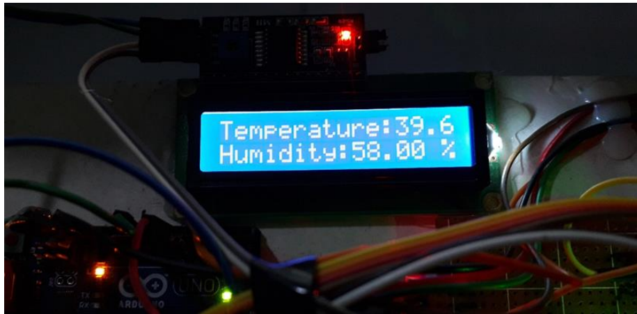
Figure 4.5.5: LCD display view Temperature & Humidity (9th place)
