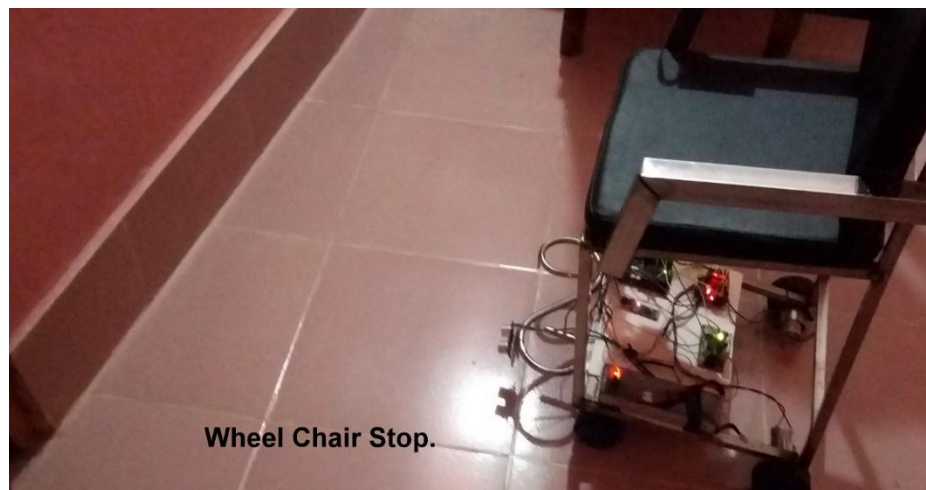
Fig. 4.11: Wheel Chair is detecting obstacles and stop.
