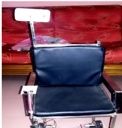
Fig. 4.12: Position of IP camera on the wheel chair.
