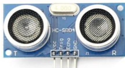
Fig. 3.8: Ultrasonic Sonar Sensor (HC-SR04). [15]
