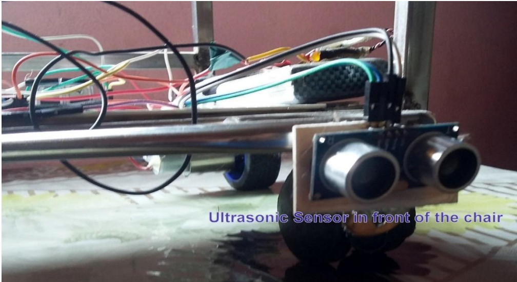
Fig. 4.3: Ultrasonic Sensor in front of the chair to detect obstacles.
