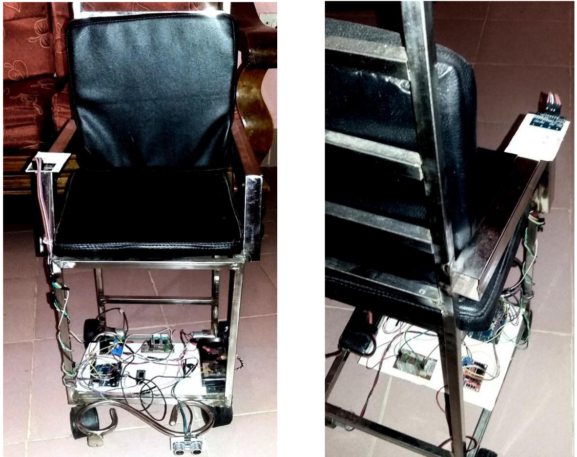
Fig. 4.1: Prototype development of Smart Wheel Chair (Front and side view)
