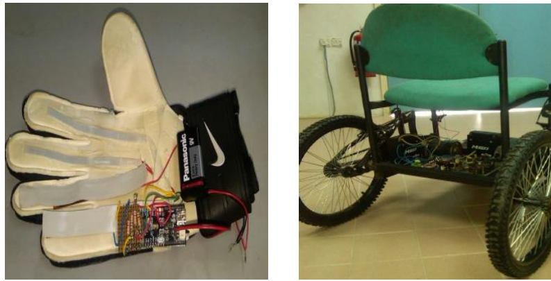
Fig. 2.5: Instrumented glove with Flex Sensor with transmitter and the prototype [1].
