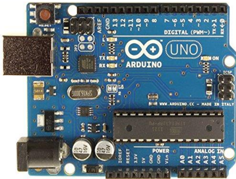
Fig. 3.3: Arduino board (UNO R3 ATMEGA328). [10]
