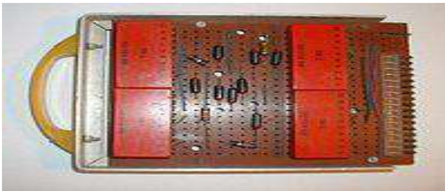
Fig.2.9 1961 Veroboard unit – components [18].
