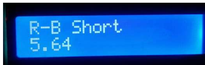
Fig 5.4 RB Short Fault Distance in Kilometer
