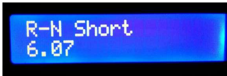
Fig 5.19 RN Earth Fault Distance in Kilometer
