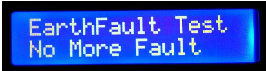
Fig 5.20 LCD Output after Resolving Earth Fault
