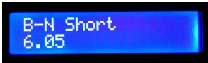
Fig 5.13 BN Earth Fault Distance in Kilometer
