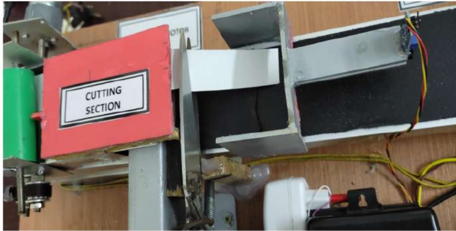
Fig. 5.10: Cutter is cutting paper
