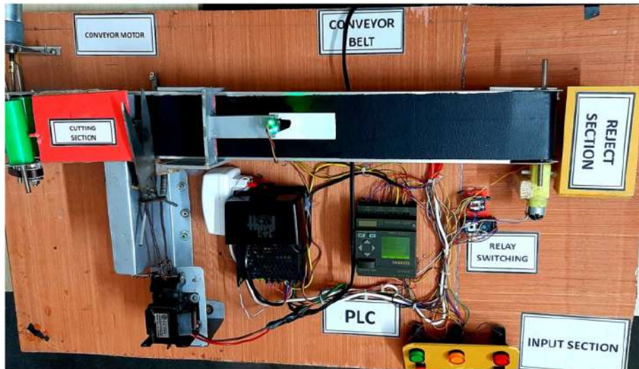
Fig. 5.11: IR Obstacle sensor measure paper size
