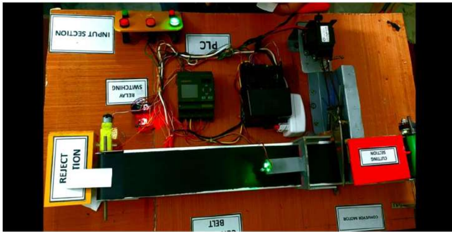
Fig. 5.13: Pass indicator is ON and paper is accepted
