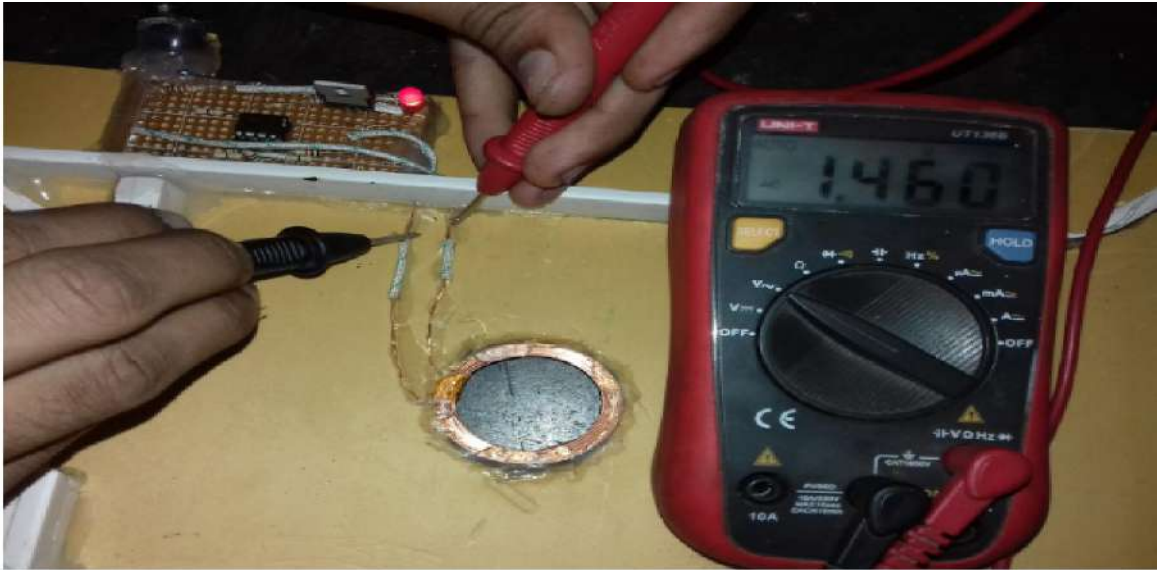
Fig. 5.7: Input voltage measuring across the transmitter side
