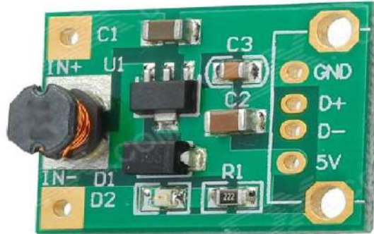
Fig. 3.9: Boost converter module [26].
