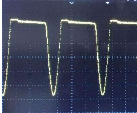
Fig. 5.13: Input wave shape of transmitting coil
