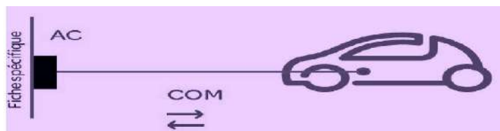
Fig. 2.7: Specific socket on a dedicated circuit [15]
