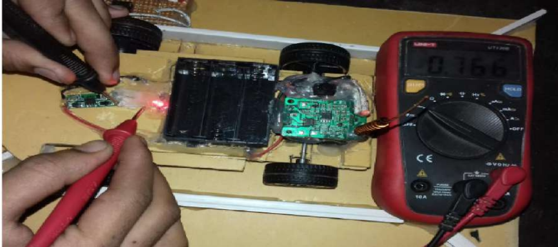
Fig. 5.9: Output voltage measuring across the receiver side
