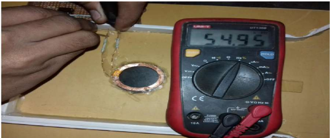
Fig. 5.8: Input frequency measuring across the transmitter side
