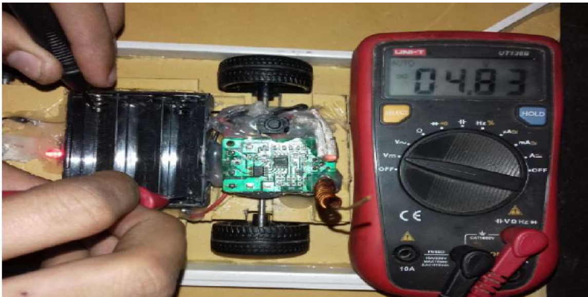
Fig. 5.10: Output voltage measuring after using boost converter
