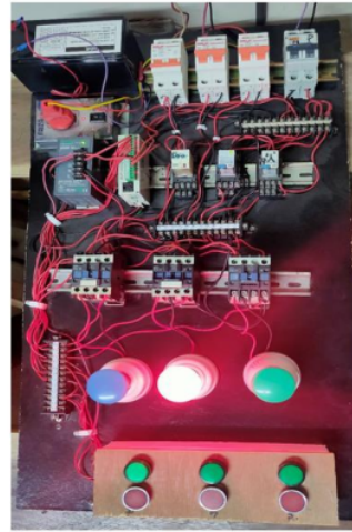
Fig.5.5: Automatic ON of Generator load
