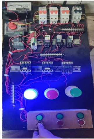
Fig.5.4: Phase Failure of PDB source
