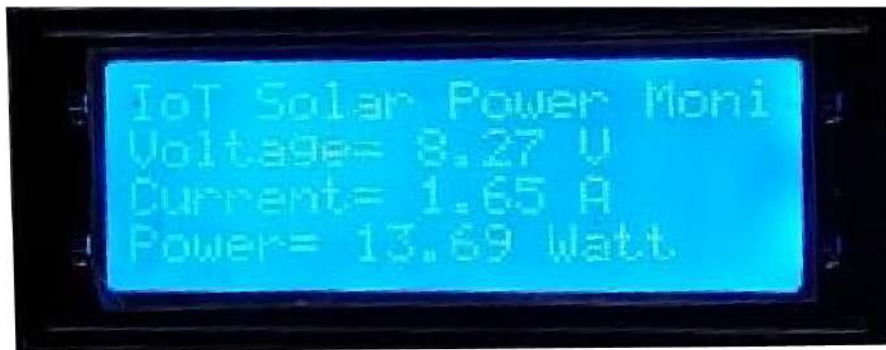
Fig. 4.19 When Load Connected, value of Voltage, Current and Power
