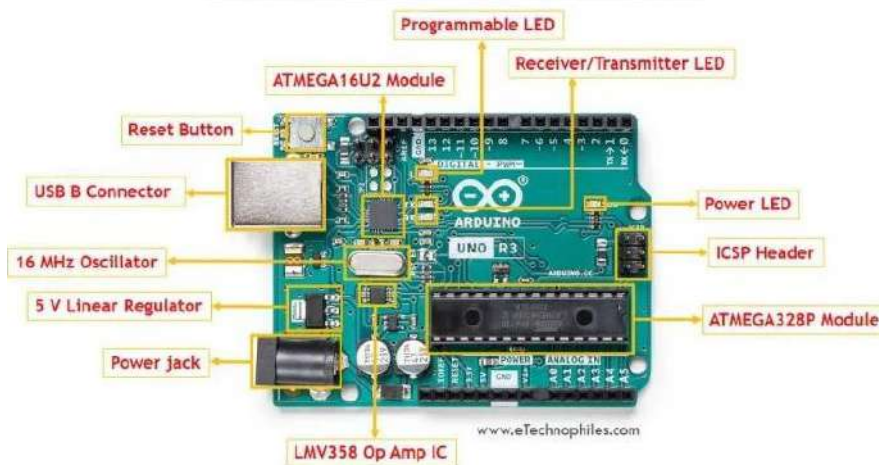
Figure 8 Layout Board of Arduino UNO
