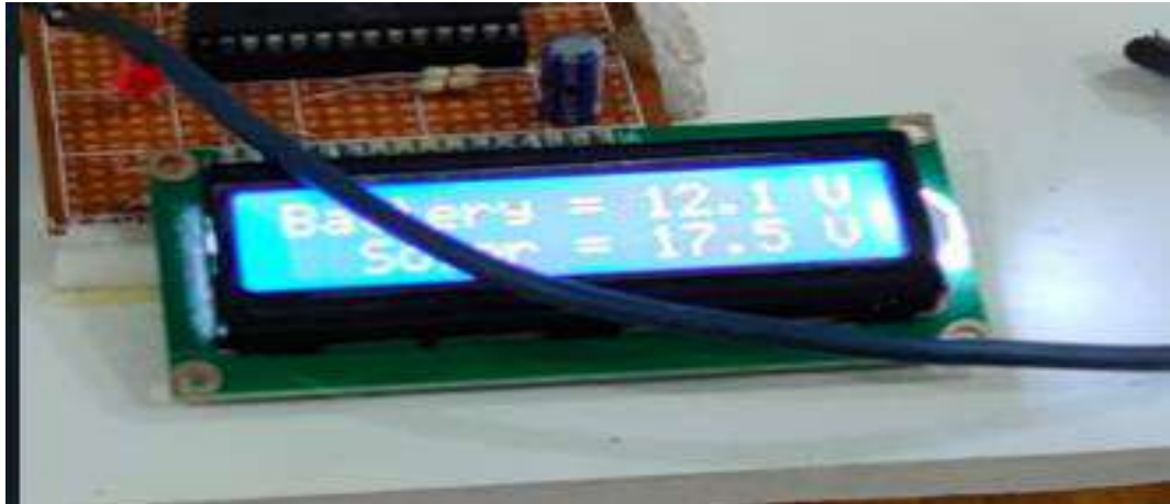
Fig 5.2: Voltage level on LCD
