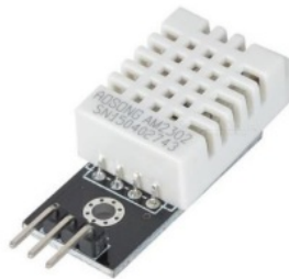
Fig. 3.8. DHT 22 Temperature and Humidity sensor [15].
