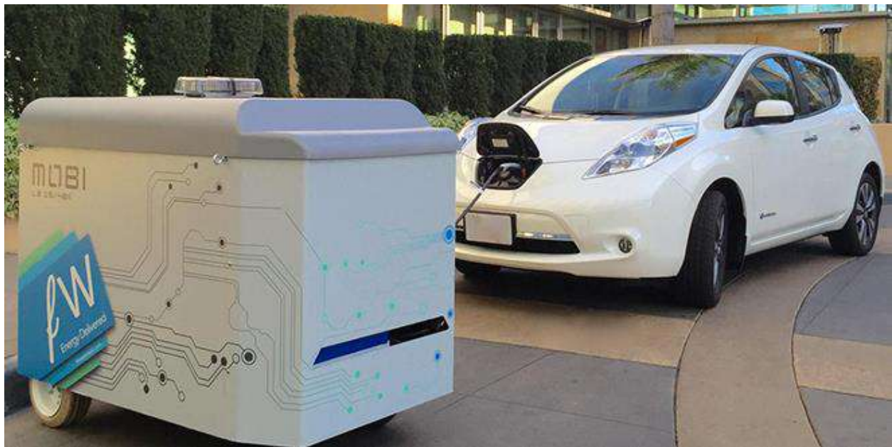
Fig. 2.5 EV charging station battery [18]
