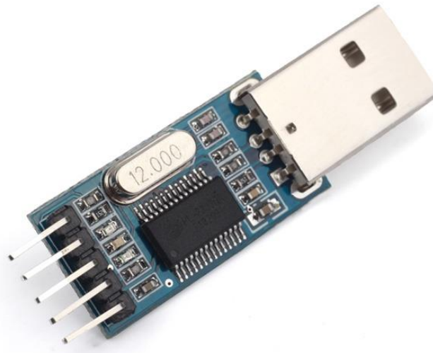
Figure-3.5: PL2303 USB to TTL Converter [16]
