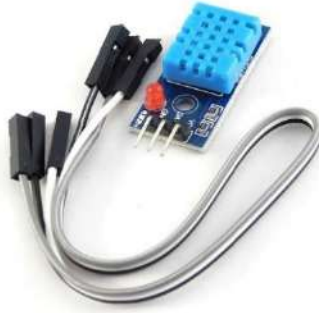
Figure 3.12 DHT -Temperature & Humidity sensor [47]
