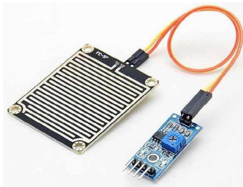
Figure 3.10 Rain Sensor Module [45]
