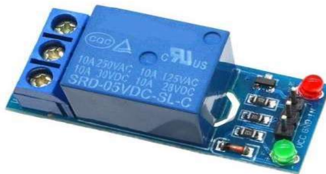
Figure 3.16 5V Single channel Relay [51]
