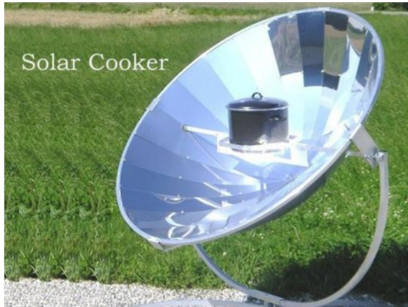
Fig: 2.1: Mirror Type Solar Cooker [3]
