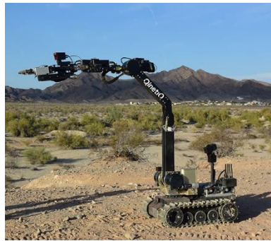
Fig. 2.1 TISON, heavy EOD robot [4].
