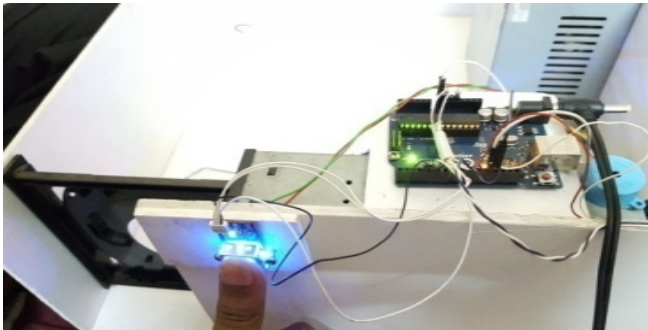
Fig. 5: Prototype of the system, finger placed on finger print scanner.
