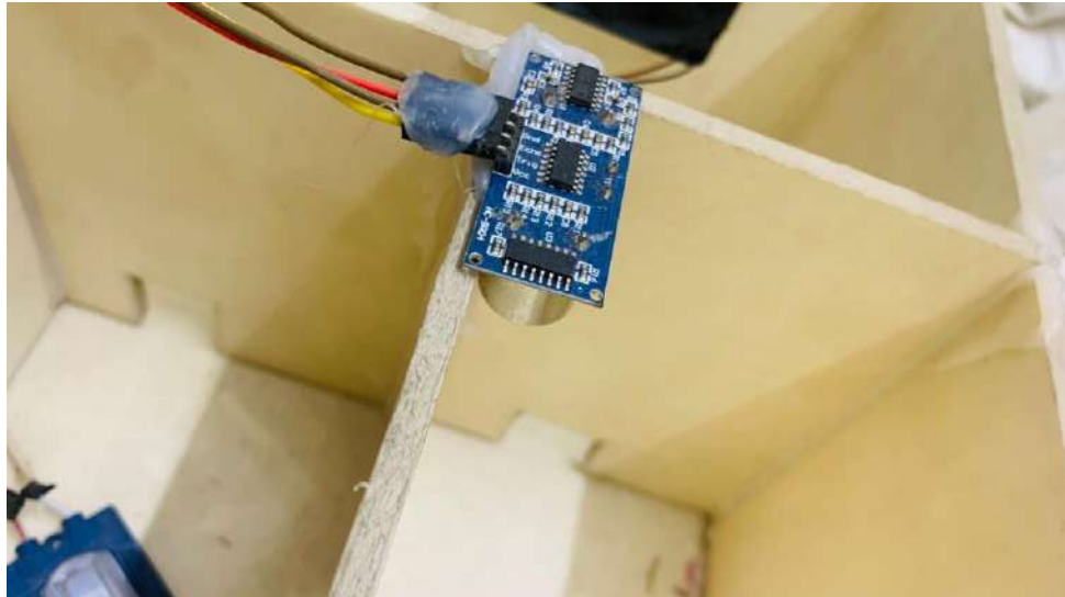
Fig: 5.7 : Sonar sensor for water level detection
