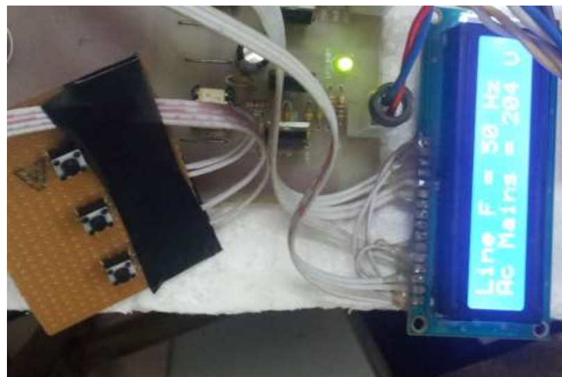
Fig. 5.8: Switching Board and LCD display
