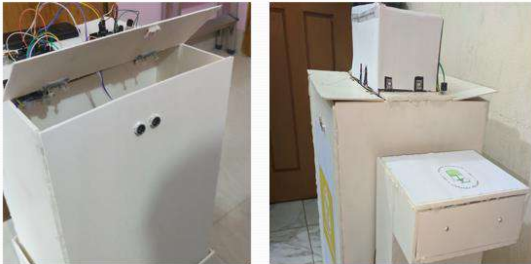
Fig. 5.2.1: Automatic Dustbin lid open and close lid system
