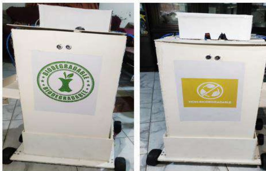
Fig. 5.2.2: Two separate chambers for Biodegradable and Non- Biodegradable trash.
