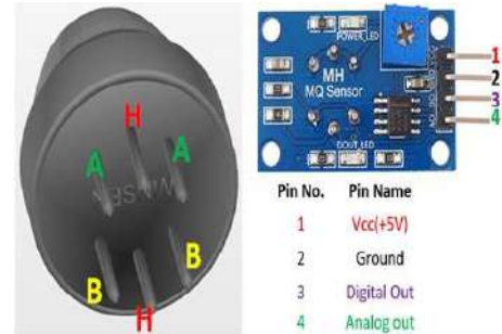
Fig. 4.11 Gas Sensor Pin out [12]
