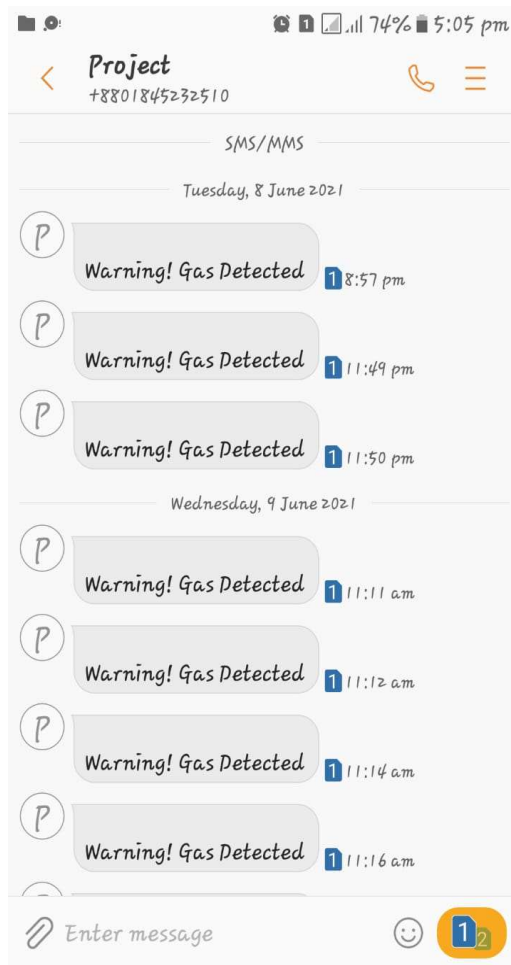
Fig. 4.2(g). Over Gas Detection Warning Via SMS
