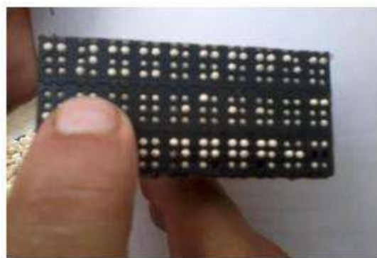
Fig 2.3: Typical Multi-Line Braille Display
