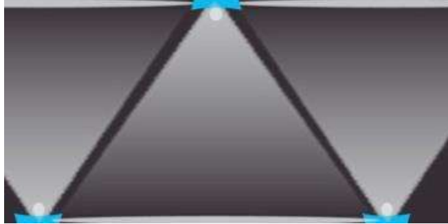
Fig.3.5.8. Angle and area are increased using concave mirror-A view from the ceiling [25]
